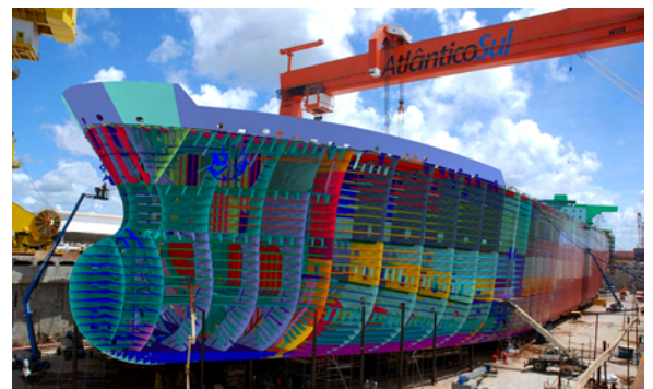
3D model of 'João Cândido', Suezmax tanker overlaid with actual vessel
