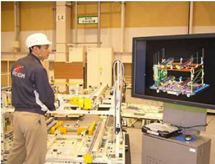
Workers do assembly using a 3D model as a guide.
