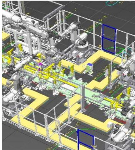
Fig.2: Mitsubishi Automobile Factory Renovation. Plant layout checked with point cloud derived via laser scanning in fall of 2010. Data input into Autodesk Navisworks.
